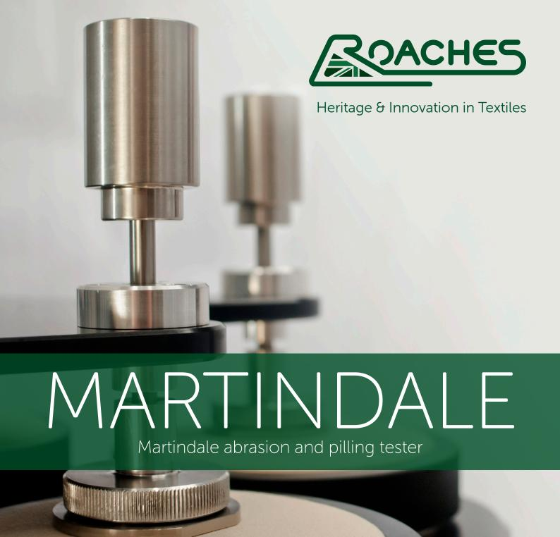
Martindale is globally recognised as a definitive apparatus for determining the propensity of a substrate for pilling and the determination of resistance to abrasion.
